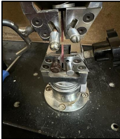
Fig. 4. A sample of acrylic that was placed into a tensile strength test
